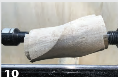
10 Complete all three twists, ensuring crisp spiral lines between them.
