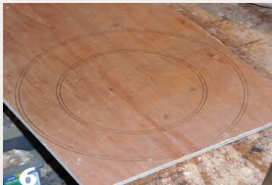
6 The inner and outer diameters of the inlay are laid out on a sheet of 6mm plywood.
