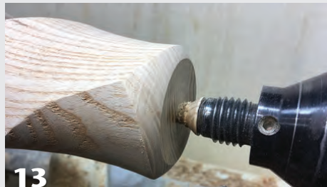
13 Shape a dome similar to the top, then cut a convex base profile, leaving a bit of the dome visible above it.
