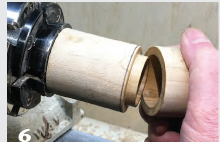
6 Cut the tenon to fit and check for a tight, flush joint.
