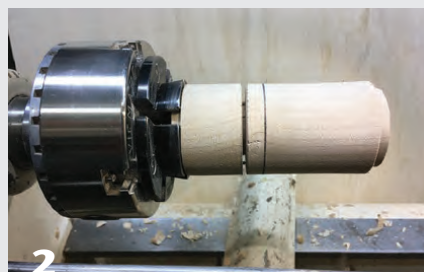
2 Mount the rounded blank in a chuck and mark the parting lines for the top and bottom.
