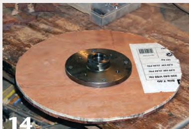
14 A faceplate centered on the plywood. The screws sit well inside the mosaic ring, so there's no risk of interference.
