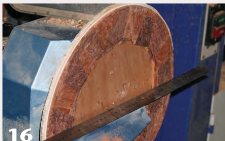
16 The author routinely checked the face of the mosaic ring for flatness until it was true.
