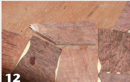
12 The fitted piece in place. Fitting is a bit of trial and error, which is why the author leaves sections oversized at the start.
