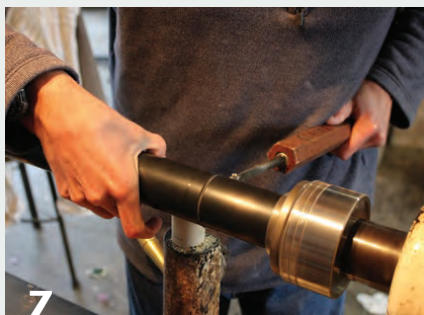
7 The ABS pipe is cut to length on the lathe with a parting tool.
