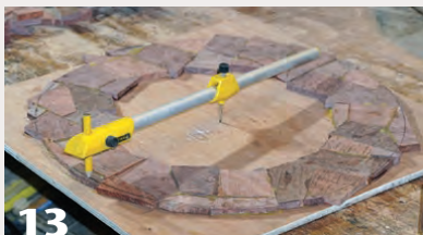
13 With the burl pieces extending beyond the original boundaries drawn on the plywood, the inner and outer diameters are redrawn onto the surface of the tiles.
