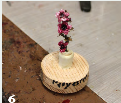
6 The base is removed from the lathe to glue the flower in place and check its alignment.
