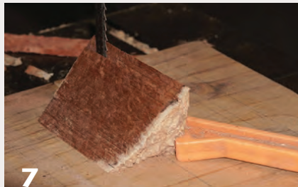
7 Triangular burl offcuts are sliced into tiles at the bandsaw, and surfaced at the linisher (belt sander).
