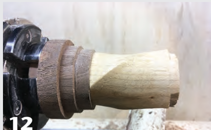
12 The author holds the box bottom in a jam chuck fitted around the outside of the tenon.
