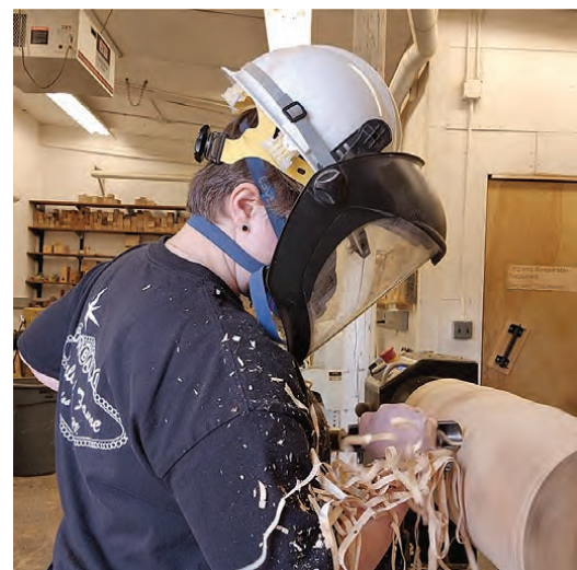
Amber Williams works on a large table spindle. PPE in turning classes includes a half-mask respirator, safety glasses, impact-rated face shield, and when warranted, a hard hat.
