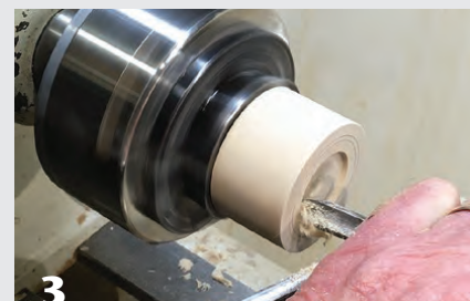
3 Hollow the lid with a spindle gouge, plunging at center and pulling toward you.
