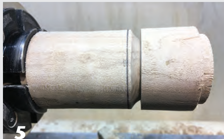
5 Twist the lid to create a burnish mark on the cove. This is your target size for the tenon.
