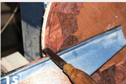
15 A small skew chisel, used as a scraper, trues the mosaic ring.
