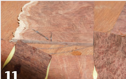
11 Marking side lengths and approximate angles on an oversized piece to fit a gap in the ring.
