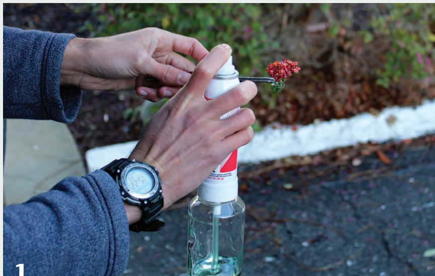
1 Spray-coating the flower with diluted resin seals the surface of the organic material before casting.
