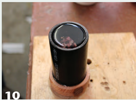
10 The slow-curing resin shows no bubbles.
