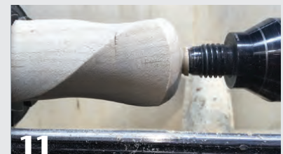
11 Shape the lid as a shallow dome, starting your cuts far enough down the twist lines for a pronounced curve where the top meets the sides.
