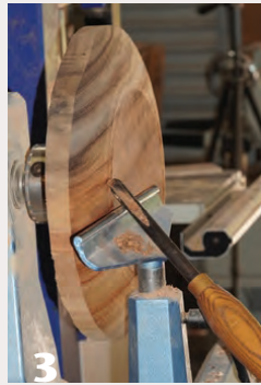
3 The author rough shapes the bottom with a pull cut.
