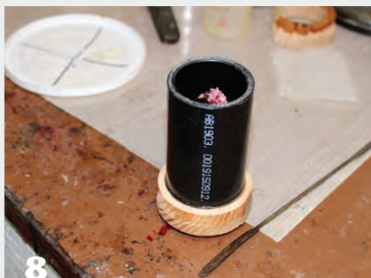
8 The completed mold is ready for casting, with the pipe seated in the grooved base and the flower in position.
