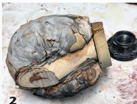
2 The author attached an oak waste block as a mount for the faceplate.
