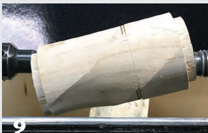
9 Check the first completed twist for a smooth, even spiral.
