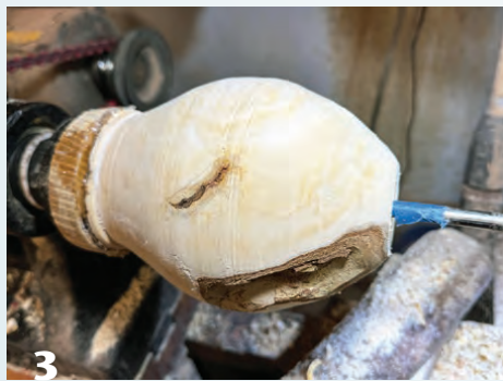
3 After shaping the exterior, a long drill bit serves as a depth gauge.
