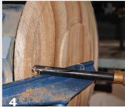
4 Then switches to a push cut to clean up the surface for sanding.
