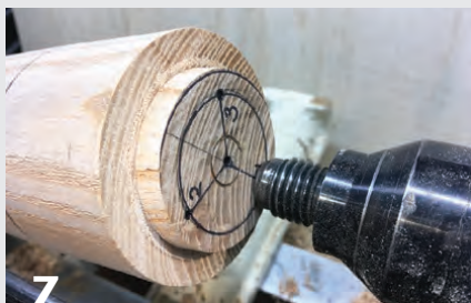
7 Mount the assembled box off-axis, with the drive and live centers seated in point 1.
