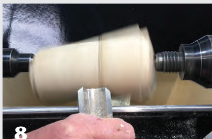
8 Set the toolrest parallel to the lathe axis and cut the first twist from end to end.
