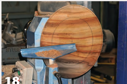
18 The camphor platter back on the lathe with the inlay dimensions transferred onto the face.
