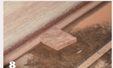
7 Triangular burl offcuts are sliced into tiles at the bandsaw, and surfaced at the linisher (belt sander).
